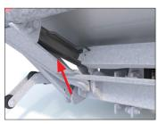
Lift cylinders store in a retracted position behind protective plating, shielding them from road debris that causes pitting.
