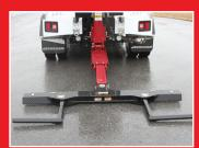
Work Confidently with a High Performing 4,000 lb Underlift that Pivots a Full 90 Degrees
