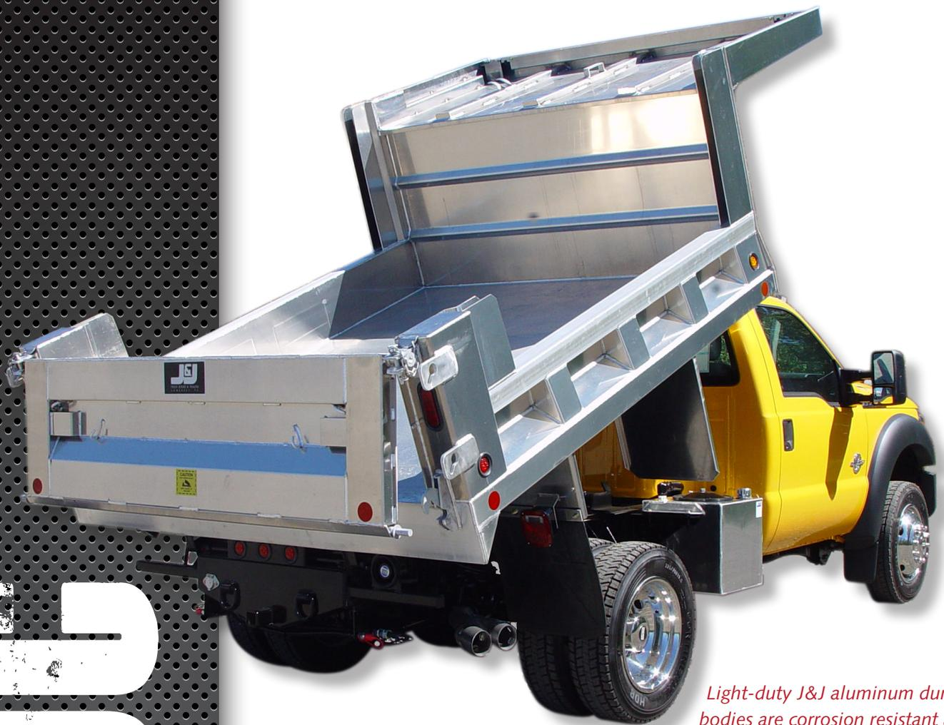
*Light-duty J&J aluminum dump bodies are corrosion resistant and lighter in weight than steel or stainless.*
