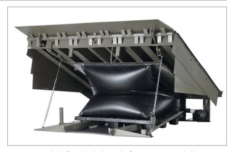
high-formed C channels for 25,000 pound Comparative Industry Rating (CIR) capacity to 40,000 pound CIR units, full length 6 inches height structural channel for 45,000 pound CIR units and full length 6 inches high structural channel and I-beams for 55,000 pound CIR units, all welded to the deck for firm structural support.
