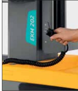
On-board charger with integrated spiral cable
