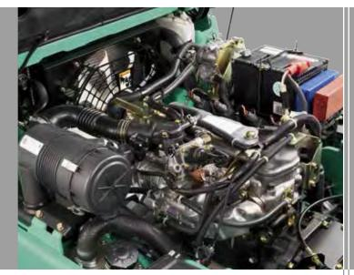
**Engine Protection:** Regulated by the Vehicle Control Module, the Engine Protection System keeps the truck running at desirable levels while helping to prevent damage to the forklift, saving you money. If any of the vital fluids becomes critically low, RPM levels are automatically lowered and the operator is immediately notified by a light on the dash display.
