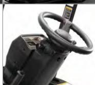
The FGC15N-FGC33N series comes standard with the Integrated Presence System (IPS), which is designed to disengage all powered travel and some hydraulic functionality when the operator leaves the normal operating position. Additionally, warning alarms sound and indicators are shown on the display panel, informing the operator and surrounding personnel that the system is engaged.
