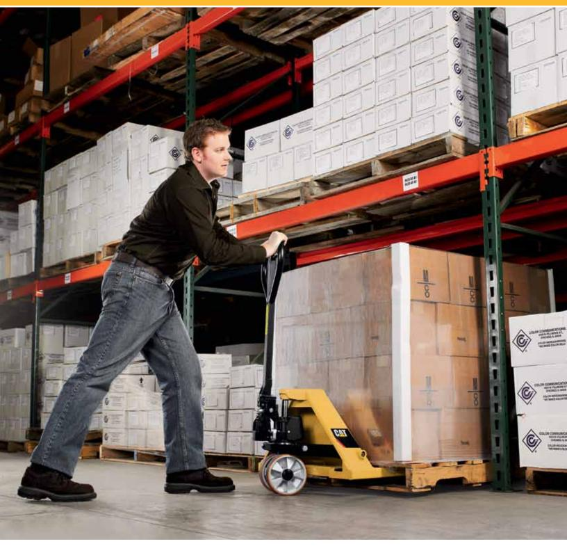
This hand pallet truck has been engineered to provide long-lasting strength and versatility.
