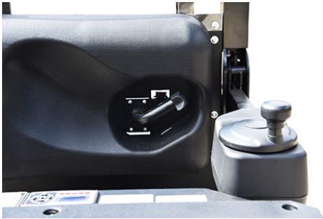
J2 -72 forks trailing controls are built in to the operator compartment backrest and activated by a laser which confirms operator hand position.
